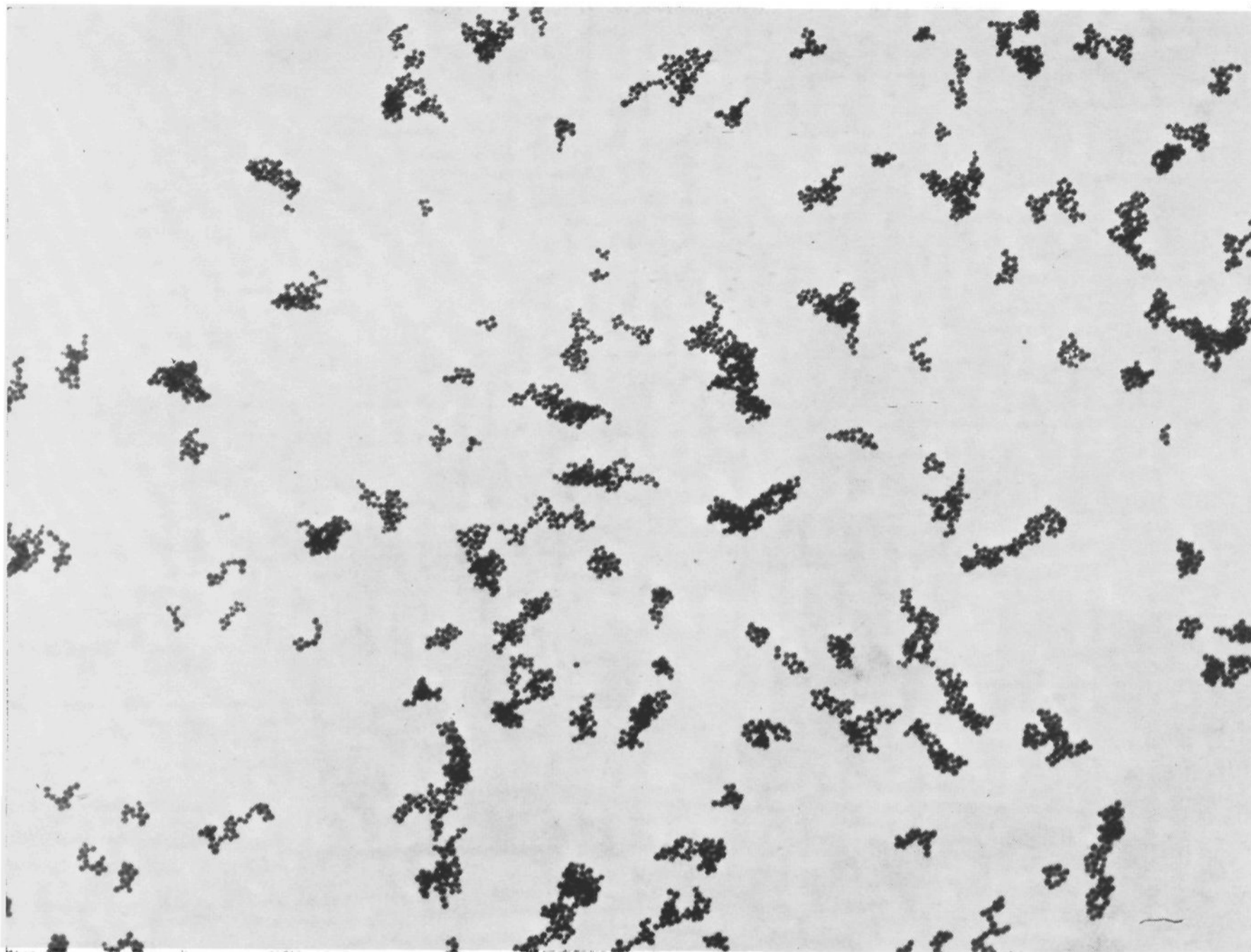
Fig. 6.—Aggregates formed by fast coagulation of colloidal gold containing 10^{-5} M sodium citrate, by 30 mM \text{NaClO}_4 ; time of coagulation, 1 hr. Note dark regions where individual primary particles are indistinguishable. They are the regions of three dimensional formation. Magnification 60,000 \times .
